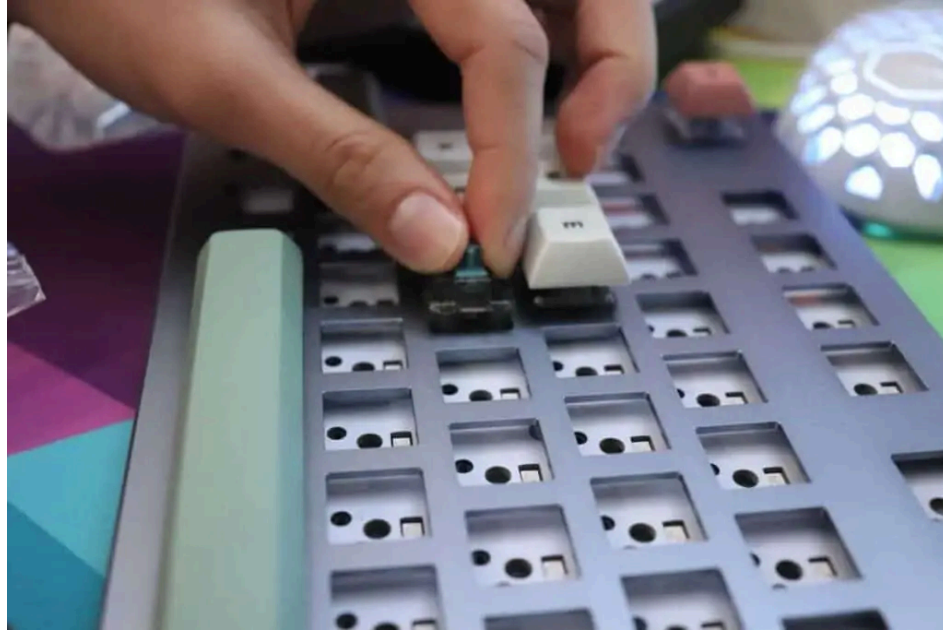
Figure 2. Switches mounted through a plate, on top of the PCB. (Source: https://switchandclick.com/plate-mounted-vs-pcb-mounted-keyboard/ )
