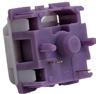
Figure 1. The bottom side of a KTT Hyacinth switch, showing straight two pins. (Source: https://www.thockking.com/products/ktt-hyacinth-switches )
